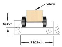
The ramps will be made from 8' lengths of 1"x 4" pine lumber with 1"x 2" side guides.
